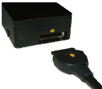
Figure 2, Aligning the USB Cable
